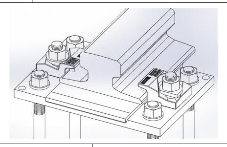
The convex in the cross-section of THRAIL resilient rail pad can make the pad carry stress reasonable. The ductile small rectangular stripes above the pad not only make the close contact between pad and rail track, but also strengthen the resilience of the pad, which can help to buffer the shock from the rail shake.
